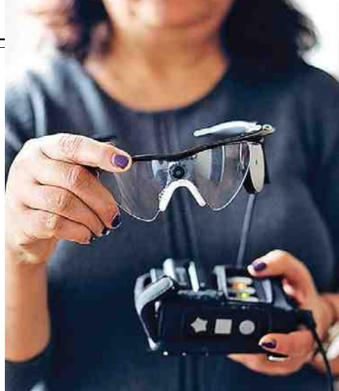
The Argus sends data from camera-equipped glasses to a retinal implant.
